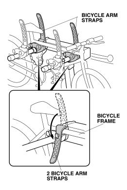
4. Install the two anti-sway straps. Tighten each anti-sway strap securely around the bicycle frame.
